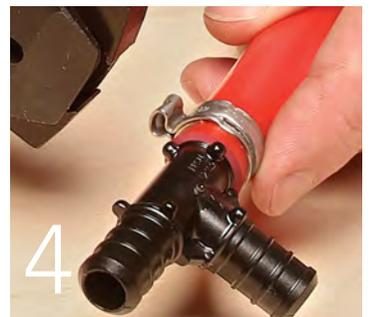
4 Place the tool's jaws over the clamp's tab, and squeeze until the tool releases. A mechanism prevents the tool from releasing until the connection is complete.
