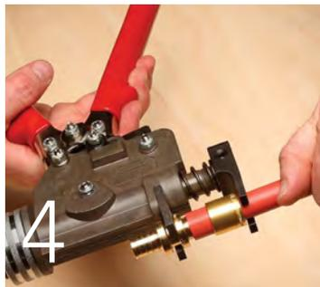
Turn the tool around and slide the compression jaws onto the fitting and tubing. Squeeze the handles repeatedly to pull the compression sleeve over the fitting and complete the connection.
