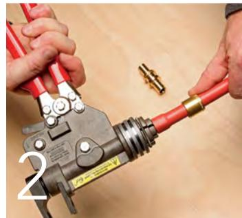
2 Insert the expansion-tool head into the tubing, and expand it. Release the tool, rotate it 45°, expand the tubing again, and hold it for five seconds.
