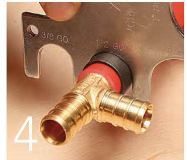
4 After crimping, check the result using a go/no-go gauge. If the go/no-go check fails, cut the tubing just beyond the end of the fitting, and start over.
