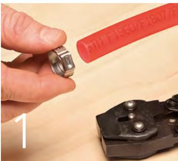
1 Slide a stainless-steel clamp onto the tubing.
