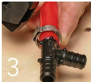
3 Align the clamp so it's about 1/8 in. to 1/4 in. from the end of the tubing. As with crimping, the clamp should be aligned over the fitting's central ribs.
