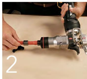
2 Insert the expansion-tool head into the tubing, pull the trigger to expand once; then rotate the tool slightly and expand again.
