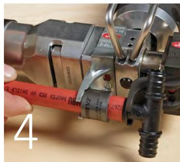
Turn the tool around and slide the compression jaws onto the fitting and tubing. Pull the trigger to pull the sleeve all the way to the fitting's collar. The tool stops and resets automatically.
