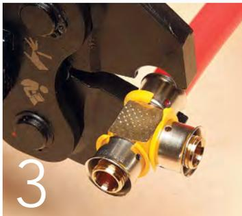
3 Align the PEX press tool squarely over the fitting sleeve.
