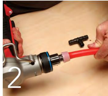
2 Repeat the expansion process until the tubing and ring butt up to the shoulder of the expansion head.
