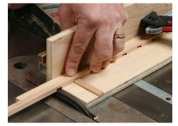
**Grid magic.** After cutting the gridwork strips to fit the opening, cut half-lap joints with a stacked dado set. A jig assures even notch spacing; just bump the tip of the workpiece against the key for the first notch, and hold it securely to the jig to make the cut. The rest index off the previous notch.
