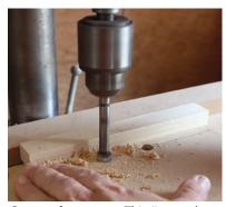
Get ready to rout. This jig needs two mortise slots. Lay out the slots, marking the centerline and ends of each slot, and then drill 3/4-in.-dia. holes at the left end of each slot. For the middle and top rails, make a similar jig with one slot for the single tenons in those joints.
