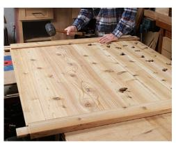
Assemble in stages. Start by inserting the panel boards into the lower and middle rail, with no glue—but fire a single brad through the rail into each board to keep it roughly in place. Then apply glue to all of the mortises and tenons and add the top rail and stiles. I used bar clamps to draw the joints home, as they get pretty snug once glue is on them.
