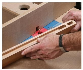
**Don't forget the grooves.** Cut all the panel grooves on the router table with a ½-in. bit, using two passes to reach the full depth. To groove the lower sections of the vertical frame parts, start the bit in one of the mortises, and rout until you reach the next one. The grooves on the rails run straight through, so they are even easier.
