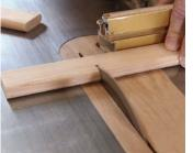
**Chop and bevel.** Cut the tenons a little short to leave room at the bottom of the mortises for the glue that will be pushed down there during assembly. Then bevel the ends a little to make it easier to insert the tenons.
