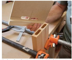
**Foolproof results.** Vacuum out the last of the wood chips, and the mortises are done. Note the long clamps used to hold the workpiece vertically against the edge of the workbench.
