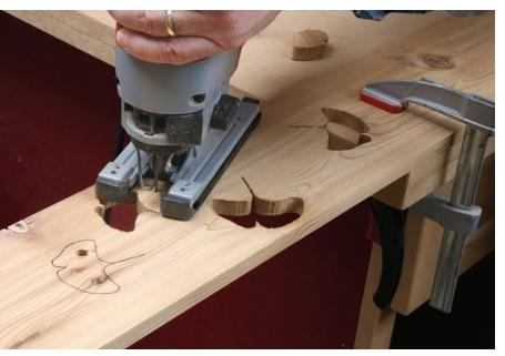
**Jigsaw does the job.** Drill holes inside the perimeter of each leaf outline to make a place to start each cutout. Then put a curve-cutting blade in your jigsaw (I used a Bosch T119BO blade), and get to sawing and sanding.
