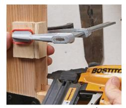
**Get ready for the gridwork.** Use <sup>1</sup>/<sub>4</sub>-in.-thick strips behind and in front of the gridwork to secure it in place. L-shaped stops help correctly locate the back strips, and shooting 18-ga. brads through the strips locks them in place.
