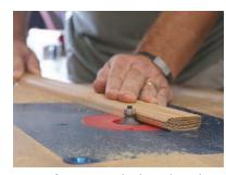
**Rip and rout.** Rip the board on the tablesaw to just narrower than the width of the mortises, then use a <sup>1</sup>/<sub>4</sub>-in. roundover bit to rout all four edges.
