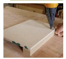
Nail on the plate. It can be difficult to get the wood fence flush with the 1/4-in. MDF. Instead, attach it so that it sticks out a little from the plate. Because the jig's fence will ride the router fence when you cut the slot, the slot will be perfectly parallel to the jig fence, which is what matters.
