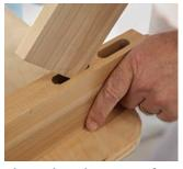
Plane a board to a snug fit. Run a board through your planer until it will slip into the mortises with hand pressure.
