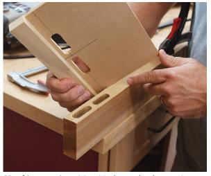
**Matching mortises.** It's critical to make the mortises in the correct locations on each piece to keep the gate square. The jig's job is to ensure that the mortises match.
