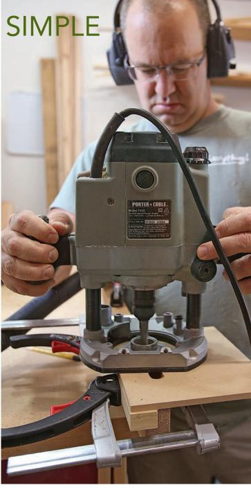
passes with a ½-in. bit. Drop one of the drilled holes over the bit to help you set the fence accurately to one edge
