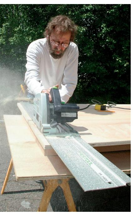
he first kitchen I ever built was a modest set of boxes made from hardwood-veneer plywood. To break down the 4x8 sheets into usable cabinet components, I used an equally modest tool setup: my circular saw, a level for a straightedge, and two spring clamps. The level made a respectable straightedge for guiding the saw, and the clamps could hold it in place. But accurately positioning the level and getting clean crosscuts time after time was a little more challenging.
