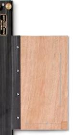
You provide the carriage's ¼-in. piece of plywood and plunge the blade through for a zero-clearance cut.
