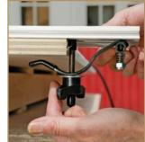
Sturdy connection. The edge guide comes in 50-in. lengths that are connected for longer cuts. The connector rods are beefy for a secure, no-slop fit. You'll need to have an Allen wrench handy, but that's the only drawback. Wing-nut clamps slide into position and operate smoothly.
