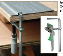
**Everything works** together. The unique design of the Festool circular saw allows it to tilt on a bevel and still cut on the same line as a square cut (top photo). Differentlength fences can be connected with rods that slide into channels (photo far left). The channel also provides a place for a clamp to secure the fence to the work (bottom photo). If you are in a hurry or use the router attachment
