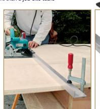
**Clamps cost extra; fence connections are easy.** You have to supply the clamps for the Tool Trolley, but the offset carriage means that they won't get in the way. Thanks to registration pins on the connector plate, fence sections are coupled quickly by tightening a pair of setscrews.
