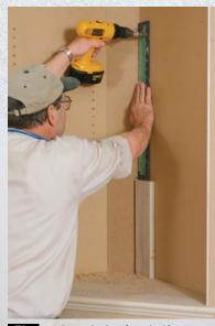
**Tip** To bore holes for shelf-support pins, I use a self-centering bit and a drilling jig from Rockler (\$27; www.rockler.com).
