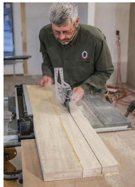
**Rip the right width.** Run the glued-up bottom rail through the tablesaw, set just a bit wider than the final width. Use a hand plane or a hand-held power planer to flatten the rail to its final dimension.
