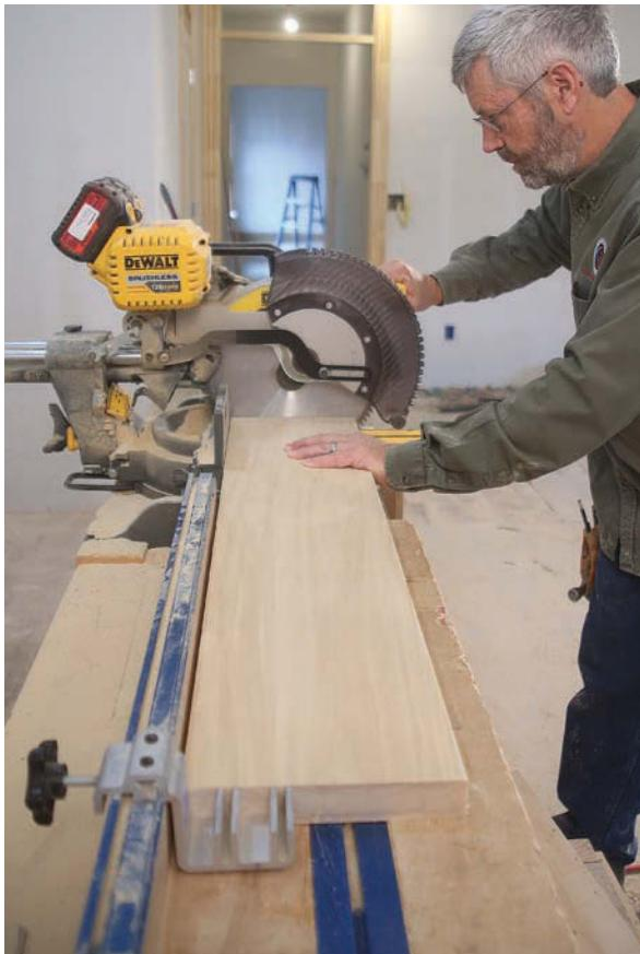
**Use a stop.** When cutting multiple parts to the same length on the miter saw, use a stop to ensure consistency.
