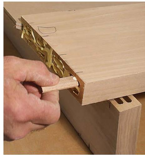
**Glue everything.** Put some glue into each mortise before inserting the loose tenons. Then add some glue to and around the tenons before attaching the outer stiles.
