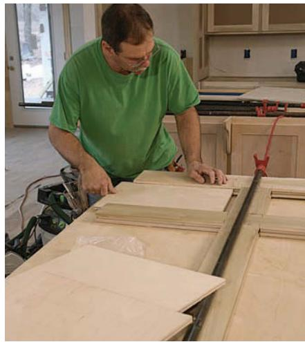
**Start in the center.** Begin by assembling all of the intermediate stiles and the rails, then slide the panels into place.
