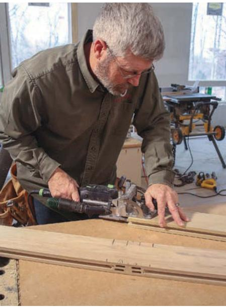
**Dominoes for days.** Cut mortises for four loose tenons in all of the joints except for the tall bottom rail. There, cut six.
