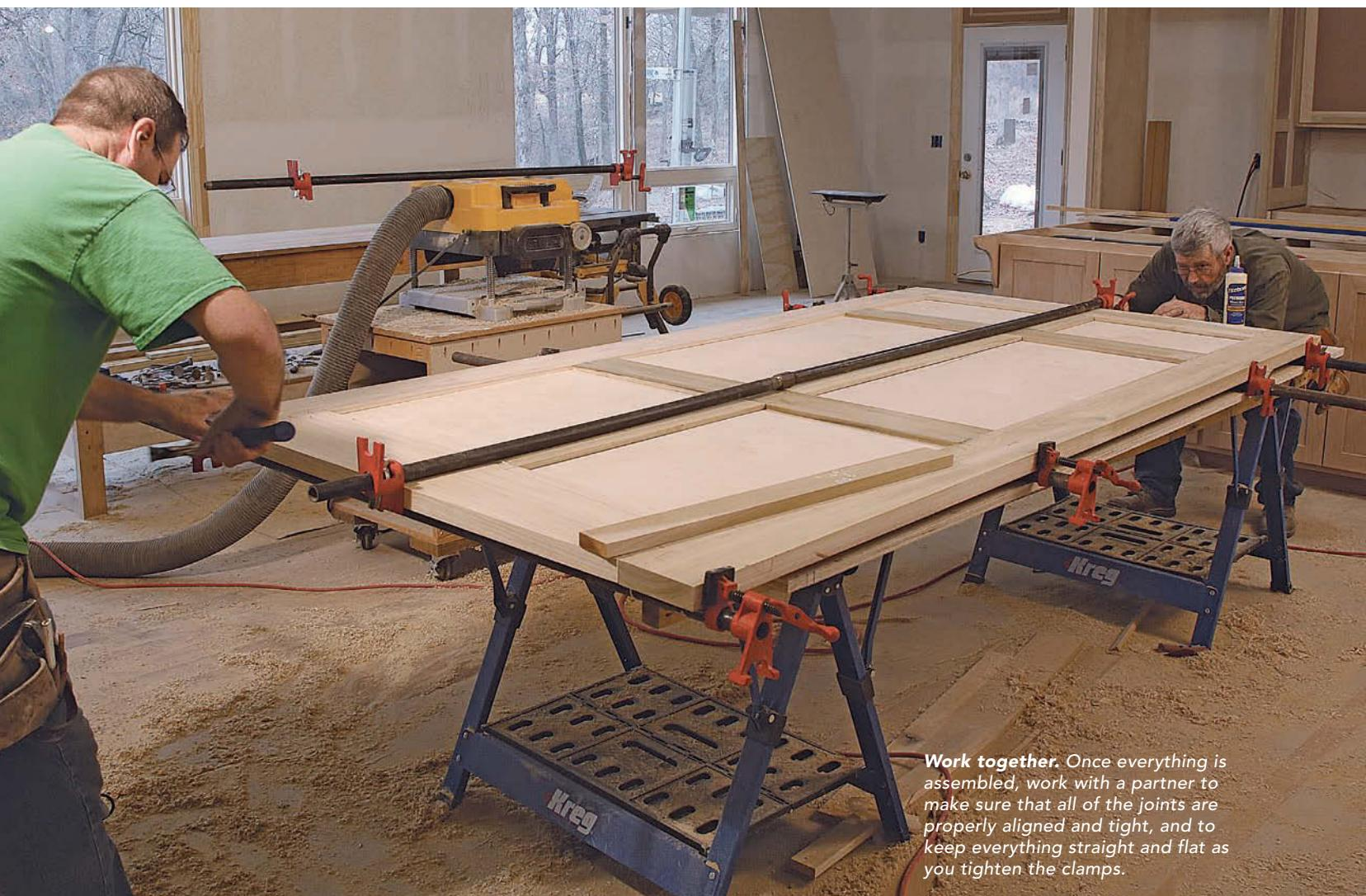
**Work together.** Once everything is assembled, work with a partner to make sure that all of the joints are properly aligned and tight, and to keep everything straight and flat as you tighten the clamps.
