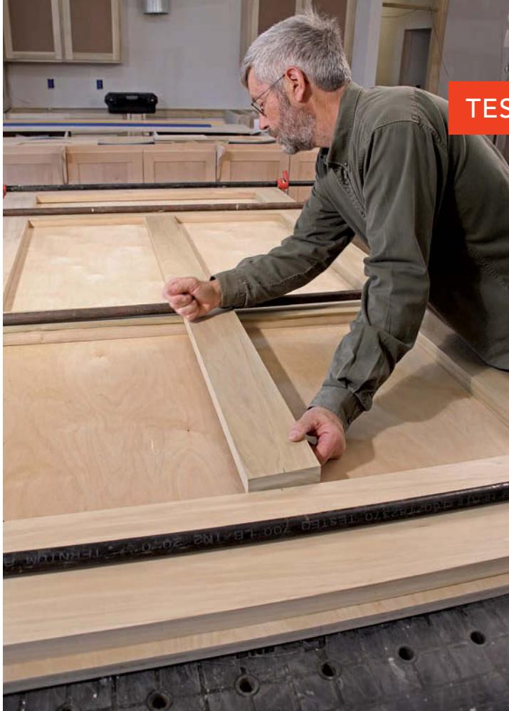
**Mock it up.** With all of the frame parts ready to go, assemble the door on a table and temporarily clamp everything in place for a test fit.
