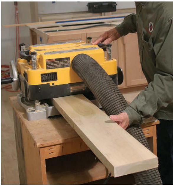
**Surface, then thickness.** Run all of the rough-cut stiles and rails through the planer, taking  $\frac{1}{16}$  in. off of each face. After everything has been surfaced, set the planer to the final thickness and run each part through again. For consistency, don't change the planer settings until everything has been cut to the final thickness.
