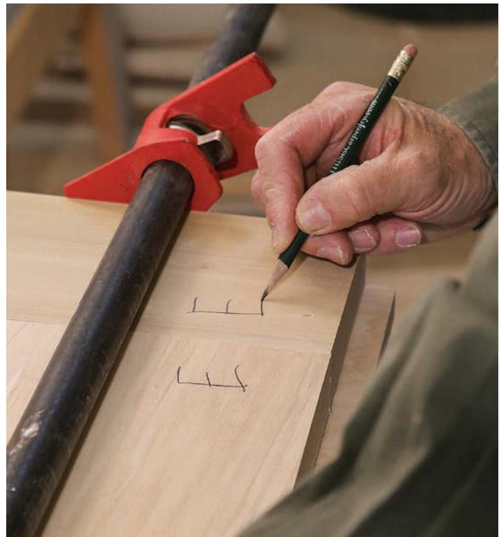
**Label the joints.** Once you have everything fitting well, letter both pieces of each butt joint to make sure that you reassemble the door the same way when it comes time for the final glue up.
