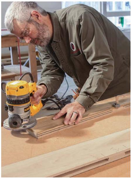
**Three passes with the router.** The panel grooves are made with a  $\frac{1}{4}$ -in. slot-cutting bit in a router. You'll need to make one pass from each side of the board and a final pass to remove the material left in the middle of the two cuts.
