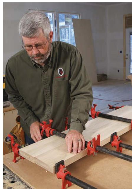
**Glue it up.** If you can't find boards wide enough to make a wide bottom rail, cut a straight edge on two boards and glue them together.
