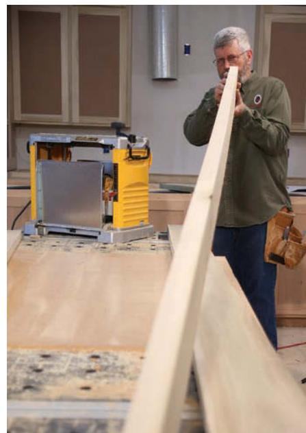
**Sort the stack.** Choose the straightest and flattest boards to use for the longest door parts—the outermost stiles. Cut the intermediate stiles and the rails from other boards. As you inspect each board, look for knots and other imperfections and keep them on the waste side of your cuts, if possible.
