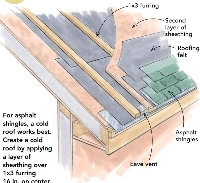
For asphalt shingles, a cold roof works best. Create a cold roof by applying a layer of sheathing over 1x3 furring 16 in. on center.
