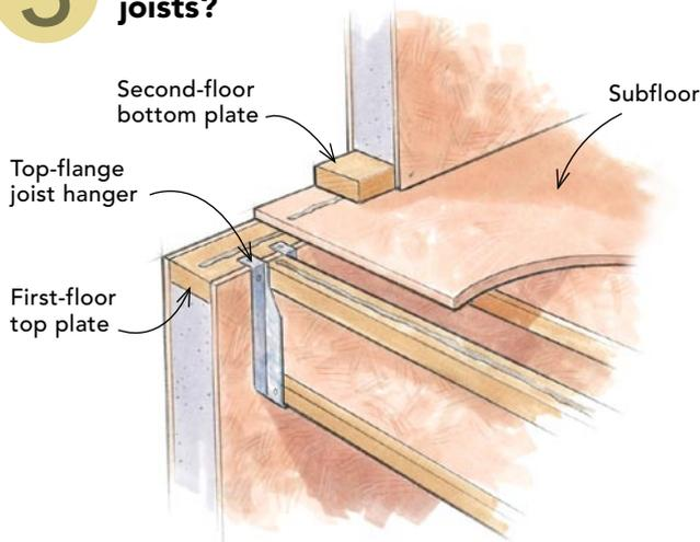
Top-flange joist hangers work in most situations. Typically, there is a 2x plate let into the top of a wall panel that is connected to both skins. The top-flange joist hanger is connected to the wall's top plate. The second-floor sheathing is installed over this connection flush with the outside skin of the wall panel.
