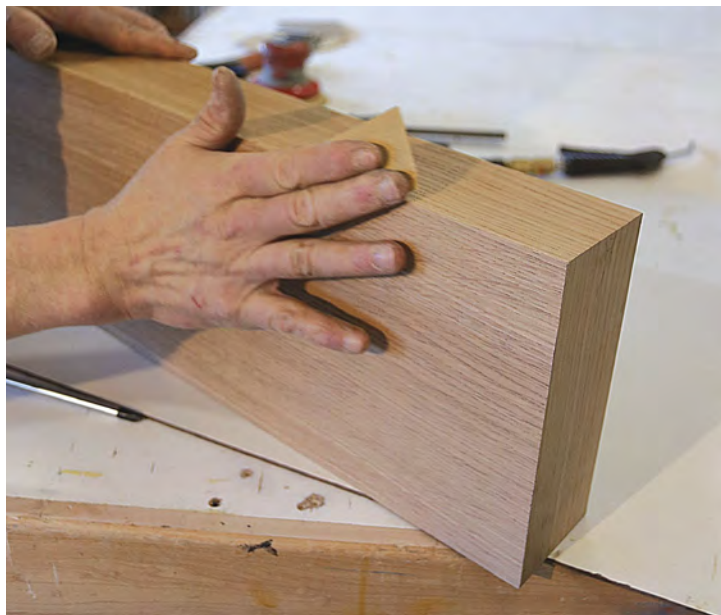
Sand lightly. Smooth the edges of the miters with 220-grit sandpaper, making sure not to sand through the veneer.
