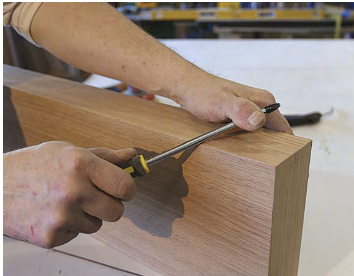
Roll the edges. Knocking down the edges with the shaft of a screwdriver makes them a bit smoother and closes any minor gaps in the miters.
