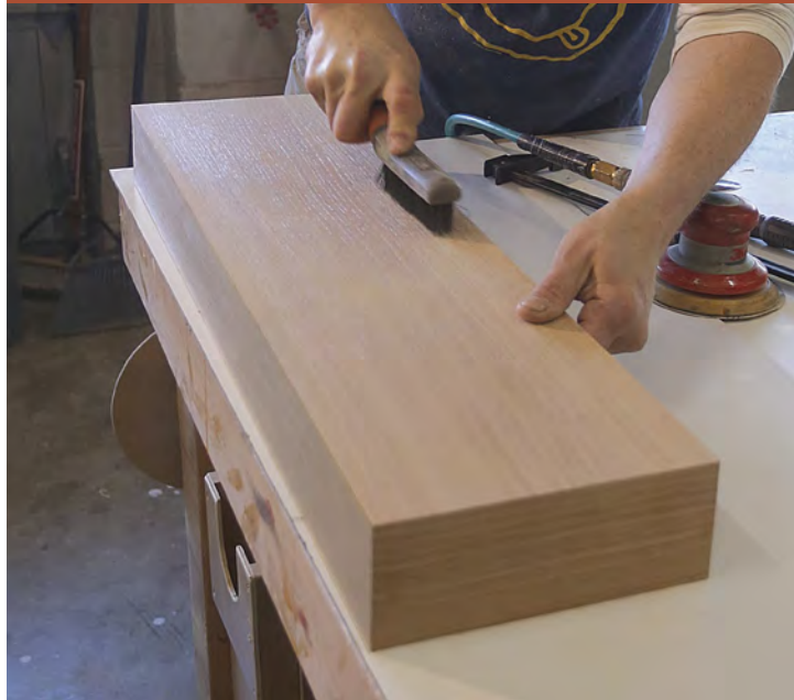
Hit it with a wire brush. A light scrubbing with a soft-wire brush raises the rift-sawn grain to add depth and texture to the finished shelf.
