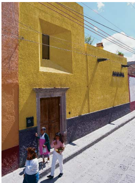
Built to the lot lines. Houses in San Miguel de Allende abut one another at the sides and are built hard against the sidewalk. This front wall of the authors' house has been rebuilt to carry a second floor, but the original front door remains. Photo taken at A on floor plan.
