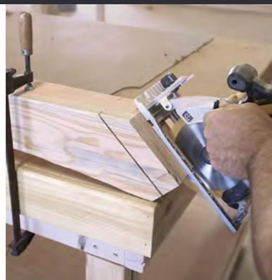
**Miter-sawn shoulder cuts.** When possible on the shorter pieces, take advantage of the accurate angles and depth of cut on a sliding miter saw to quickly define tenon shoulders. Then, the tenon can be finished up with two passes of a circular saw.
