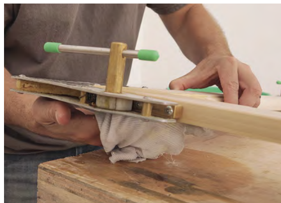
1 Don't starve. Squeeze glue into the biscuit slot and onto the face of one side of the miter, insert a #20 biscuit, and smear the glue around with a finger. There should be plenty to coat the other workpiece.
