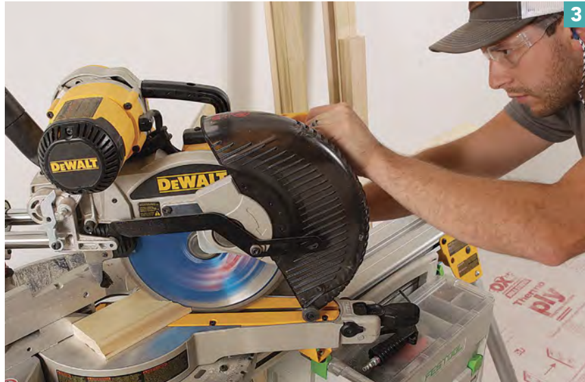
3 Kiss the line. Cut all of the left-hand miters, then swing the saw to 45° the other way to cut all of the rights. Take most of the line to ensure that the finished casing will hide the reveal marks.
