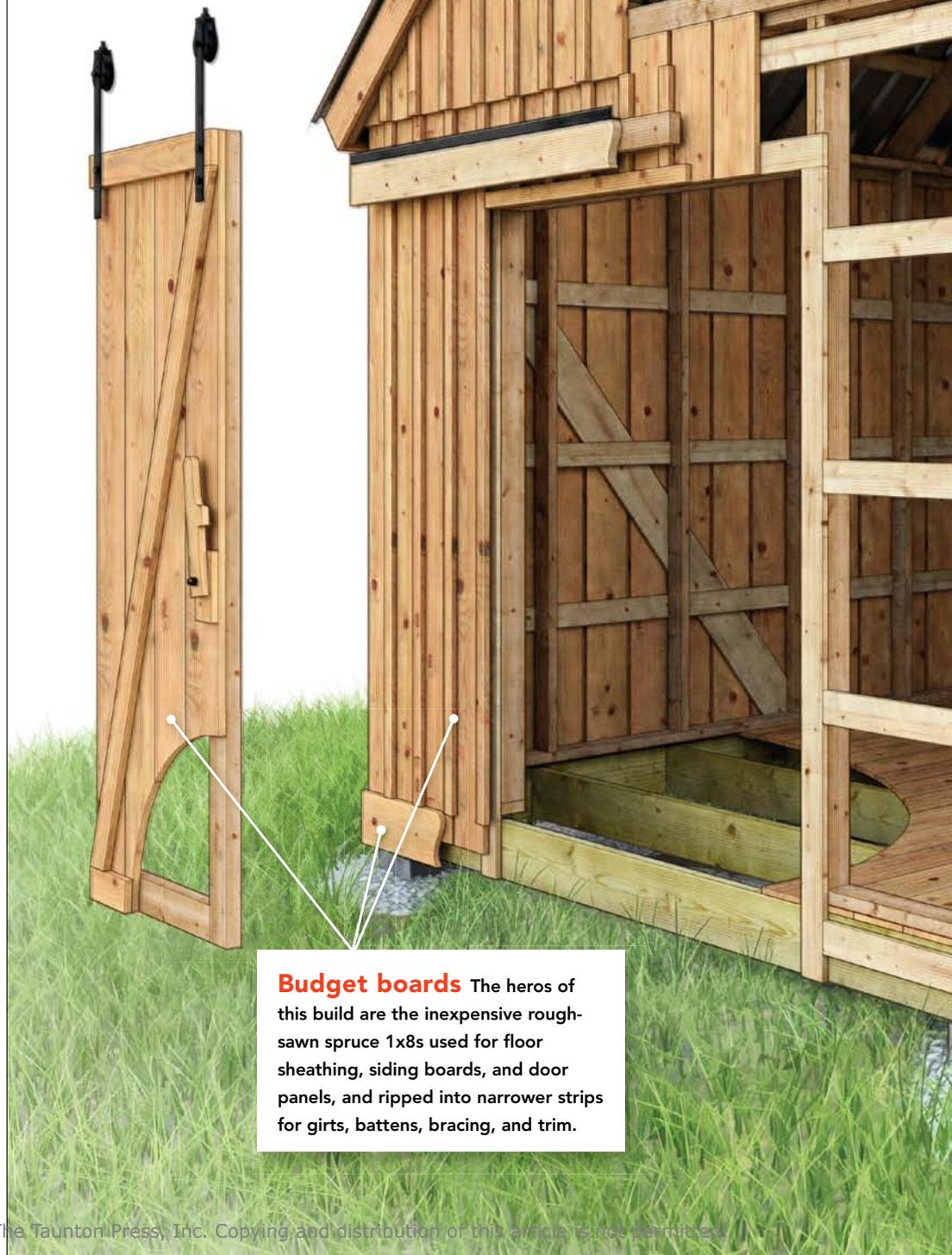
**Budget boards** The heroes of this build are the inexpensive rough-sawn spruce 1x8s used for floor sheathing, siding boards, and door panels, and ripped into narrower strips for girts, battens, bracing, and trim.
