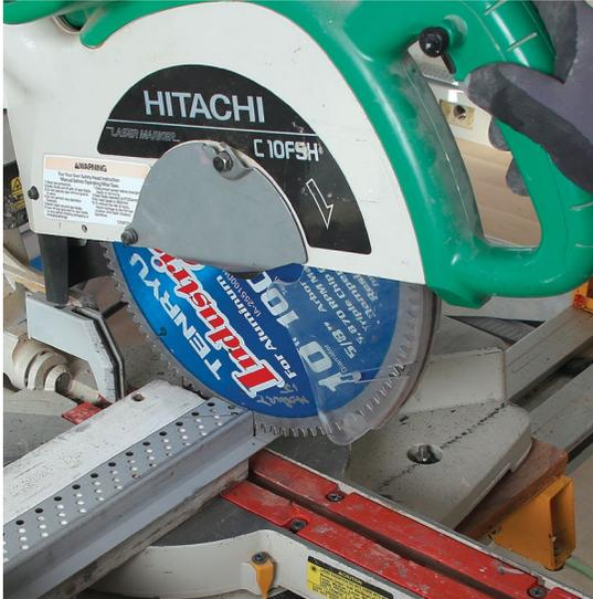
**Use a miter saw for crosscuts.** Cut metal reglet with a 100-tooth metal-cutting blade. Lube the blade with paraffin for smoother cuts, and add a piece of stock to the saw table for uniform support. Use your old miter saw; cutting the reglet is messy.
