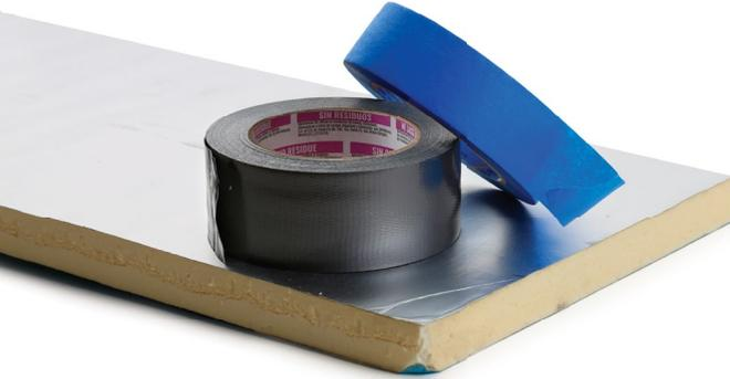
**Close the openings.** A piece of foam insulation reinforces poly sheeting to resist the pressure created by wind or a floor sander's fan. XPS works fine, but tape sticks better to foil-faced polyiso. We use painter's tape for short-term (up to two weeks) adhesion to walls and trim. We use 3M No-Residue tape for longer projects, and for adhering to sturdy surfaces like metal or trim with semigloss paint.
