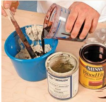
**Mix the grain filler with the stain to add color to the grain.** Follow the label directions for the proper filler-to-stain ratio and consistency. Here, I accented the grain by using a darker stain. It's also possible to use a lighter stain for a different effect.
