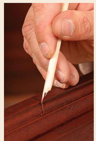
**Don't forget profile transitions.** Filler left on edges or in grooves results in a sloppy look when the piece is finished. A dull putty knife or pointed stick works well to clean these areas.
