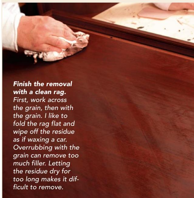
**Finish the removal with a clean rag.** First, work across the grain, then with the grain. I like to fold the rag flat and wipe off the residue as if waxing a car. Overrubbing with the grain can remove too much filler. Letting the residue dry for too long makes it difficult to remove.
