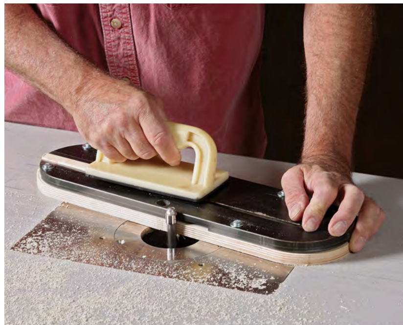
The zero-clearance route. Zero-clearance inserts are available for nearly all modern portable tablesaws, but if they aren't available for your cabinet or contractor's saw, or you just want to have backups, make a stack of homemade inserts using the existing throat plate as a pattern for cutting with a bearing-guided router bit.
