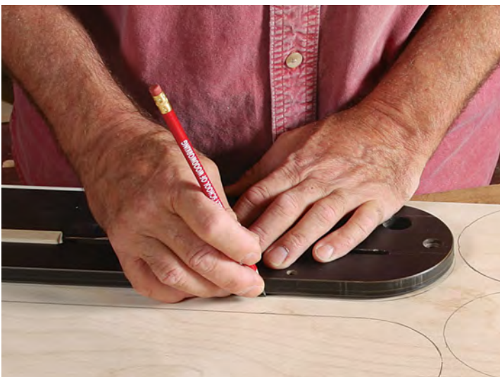
The zero-clearance route. Zero-clearance inserts are available for nearly all modern portable tablesaws, but if they aren't available for your cabinet or contractor's saw, or you just want to have backups, make a stack of homemade inserts using the existing throat plate as a pattern for cutting with a bearing-guided router bit.
