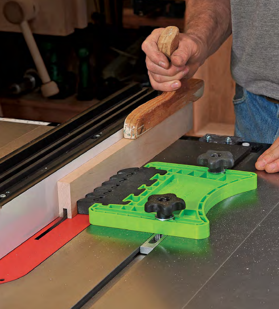
Featherboards are your friend. As extra insurance against kickback, with the added benefit of more consistent cut results, try using a featherboard. These can be site-made by cutting kerfs into a piece of scrap, but I prefer the FeatherPro, a foam-fingered plastic version that fits into the miter slot of the sawtable, eliminating the need for a deep-reach clamp.
