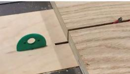
**Cure for kickback.** Riving knives are now standard equipment on saws, but older models can be made safer with the addition of a splitter like the MK splitter shown here that attaches to the saw's throat plate and helps keep material from coming into contact with the back of the blade.
