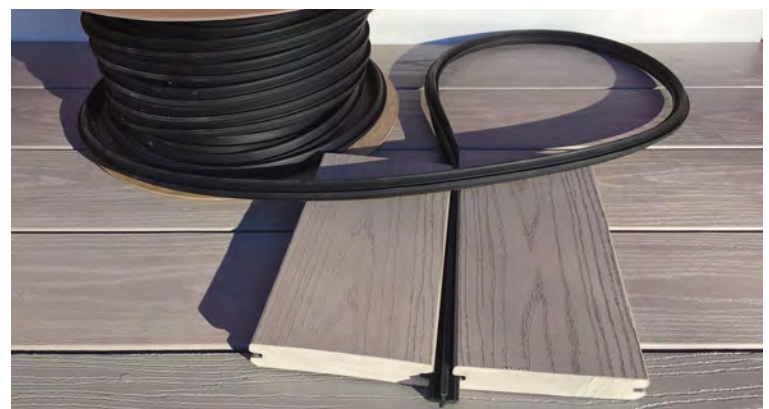
Watertight flange. Dexerdry produces waterproofing thermoplastic flanges to fit into the hidden fastener slots of various manufacturers' deck boards. More of an accessory than a system, Dexerdry also relies on a properly pitched deck for drainage.
