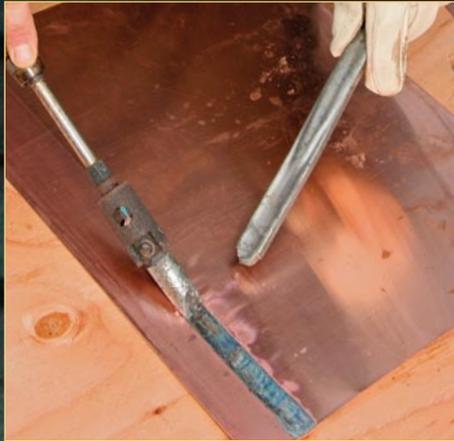
**Tin the sleeve stock.** To ensure that the solder seals the joint fully once it's formed, run a thin, smooth layer of solder along the two edges that will overlap.
