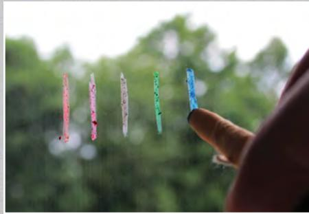
**The best by far for glass.** Wax pencils make clear marks on glass that are durable but also easily removed with solvent.
