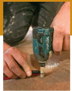
**MAKE A MARK** Place the open end of a tape-wrapped bit holder against a piece of scrapwood, hold a felt-tipped marker against it, and gently pull the trigger. As the bit holder spins, the marker creates a bold reference line. (The line's location on the holder doesn't matter.)
