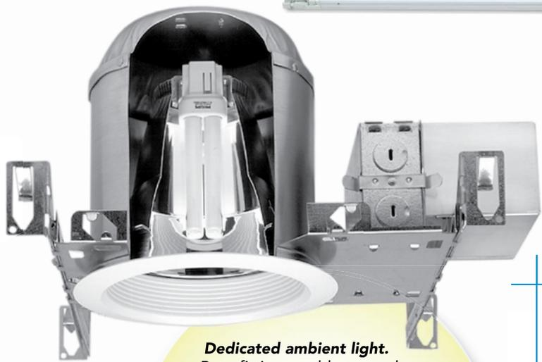
**Dedicated ambient light.** Retrofitting an old recessed can with a screw-base CFL could cause premature heat-induced bulb failure. CFL-dedicated recessed cans properly dissipate heat and maximize light output. The can above, from Halo, is remarkably similar to a standard incandescent fixture with the addition of a ballast attached to the junction box. The fixture below, from Lightlier, orients the bulb horizontally and needs just 3½ in. of clearance.
