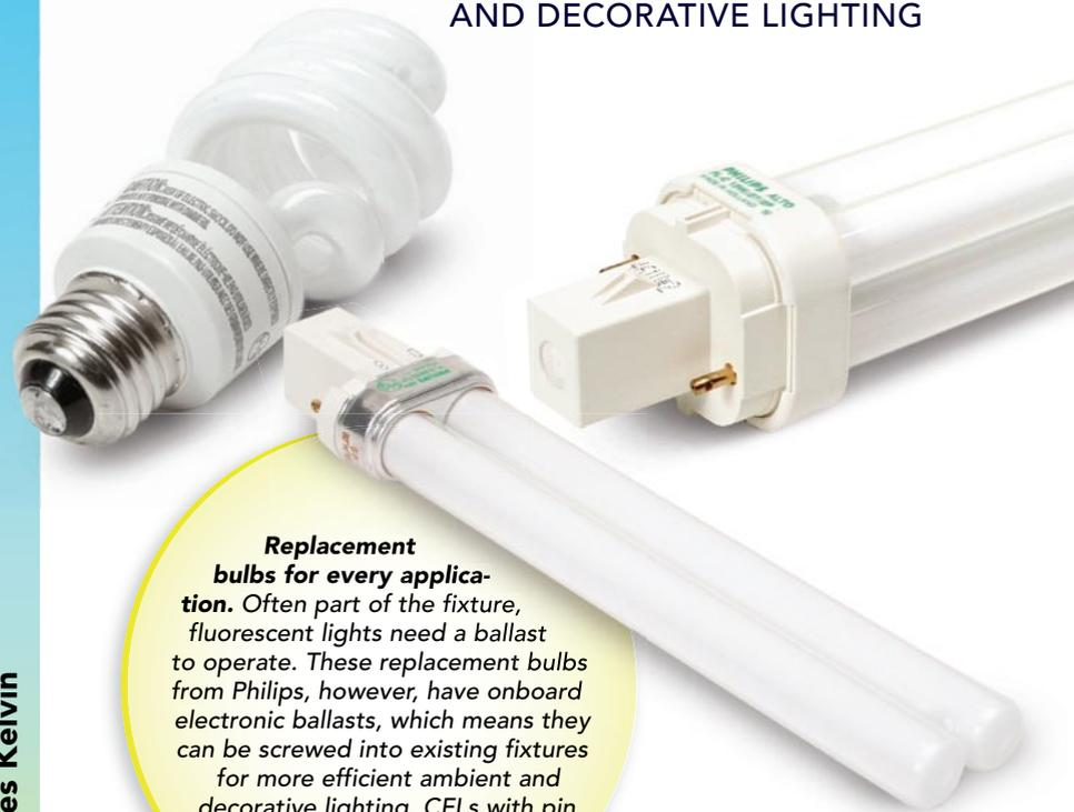
**Replacement bulbs for every application.** Often part of the fixture, fluorescent lights need a ballast to operate. These replacement bulbs from Philips, however, have onboard electronic ballasts, which means they can be screwed into existing fixtures for more efficient ambient and decorative lighting. CFLs with pin bases are for fluorescent-only fixtures required by some energy codes.
