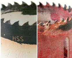
Only a few of the hole saws tested sported a finish (left) that didn't impair the speed of cut.
