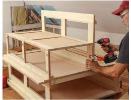
Support where you need it Blocks clamped to the vertical divider hold the web frame for the top row of drawers at the proper height. Outer supports are pocketscrewed to it and the frame below.
