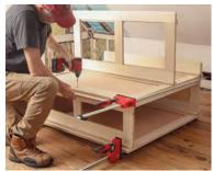
Add the second layer The upper web frames are added and incorporate a lip to support the ends of the planks that make up the bed platform.
