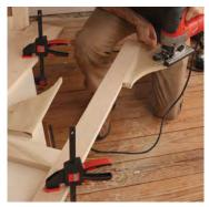
**Cut curves in place** Rectangular stock for the curved bed-rail brackets is easier to attach to the face frame before shaping with a jigsaw and sandpaper.
