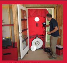
A MEASURE OF SUCCESS A blower-door test is the standard for finding out how airtight the building enclosure actually is. Some performance standards, such as Passive House, require extremely low levels of air leakage.
