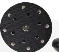
The Makita feels well balanced and has a very smooth operation. Unfortunately, it had the worst performance of the tools we tested, producing disc-sized swirl inconstancies in both the 80-grit and 220-grit scratch tests. The dust port was the smallest of all the sanders and required the most complicated adapter setup to connect to a dust extractor. The Makita has a permanently attached 96-in. cord.
