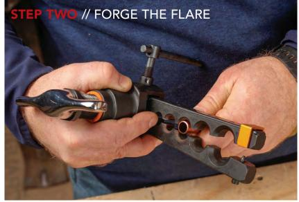
**INSERT THE TUBING** Use a flaring tool made specifically for refrigerant work to forge the flare. Start by inserting the tubing into the correctly sized hole in the block.
