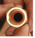
**INSPECT THE FLARE** Make sure the flare is properly sized and free of defects.
