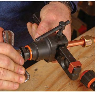
**EXPAND THE TUBING** Rotate the handle clockwise. This rolls a steel cone around the inner surface of the tubing, expanding it to the correct dimensions. A clutch prevents the cone from rolling the copper too thin.
