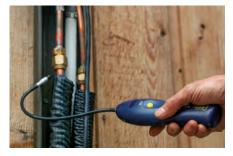
The final test is done with an **ELECTRONIC REFRIGERANT LEAK DETECTOR.** Once the refrigerant is released into the system, the leak detector is passed over flares and other fittings. This provides a last chance to catch leaks while still on-site. It also checks components like service valves and access ports that cannot be tested by other methods.
