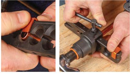
**CLAMP THE TUBING** Some flaring tools have a stop to ensure that the tubing is positioned at the right depth. Tighten the handle to clamp the tubing and yoke assembly in place.
