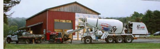
**MAKE ROOM FOR BIG RIGS** Both the concrete pump, which is pulled by a dually flatbed, and the front-discharge mixer are more than 30 ft. long, so you'll need space for them to park. Also, consider road and bridge weight limits, as a loaded mixer weighs 73,000 lb.
