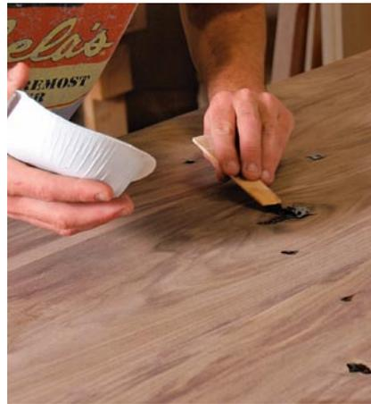
**Fill knots and blemishes with epoxy.** After scraping away any loose material, use five-minute epoxy with a coloring dye ([www.homesteadfinishingproducts.com](http://www.homesteadfinishingproducts.com)) to fill knots and other blemishes.
