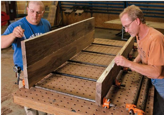
**Glue both faces liberally.** Starting about 3 in. in from the ends, space clamps every 12 in. Top clamps will be placed between the bottom clamps after the glue is applied. Start with an outside board, tip it up, and run a glueline down the middle. You can't put on too much glue, but you can use too little. Use a solder brush to spread glue.
