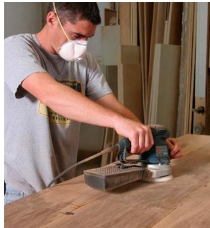
**Sand, then sand more.** With 60-grit sandpaper on a random-orbit sander, correct any cosmetic defects, paying special attention to the joints. Use a straight-edge to make sure that the top is perfectly flat. Sand with 80-, 100-, 120-, and 180-grit sandpaper. Start sanding the edges once you've gotten to the 120-grit paper. Wet the top with mineral spirits to reveal remaining defects.
