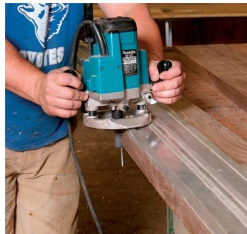
**Prepare the surfaces' mating edges.** Use a jointer or a router and guide to create one perfectly straight edge. If you use the latter technique, rip the board on a tablesaw, removing just enough material to create a parallel straight edge. Flatten the board on a jointer, and plane it to within 1/32 in. of final thickness. The remaining 1/32 in. will be removed later when the blank is sanded.
