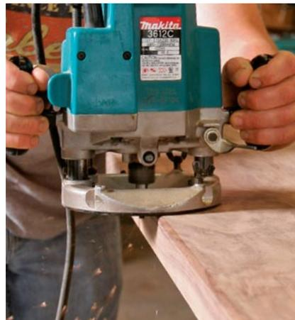
**Profile the edges.** Use a bottom-mount, bearing-guided router bit. Depending on the profile, you might need to make multiple passes. Sand the profile with 120- to 180-grit sandpaper. Soften or ease all sharp edges. Finally, sand the entire top to 220 grit.
