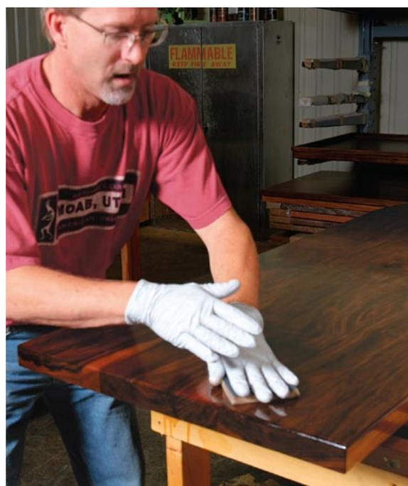
**Wet-sand the last coat.** When the counter stops absorbing the finish at a dramatic rate, likely by the third coat, apply the finish, and wet-sand it with fine foam sanding pads. Once you've sanded the entire top, wipe off the excess finish. Use a power buffer to bring the finished top to life.
