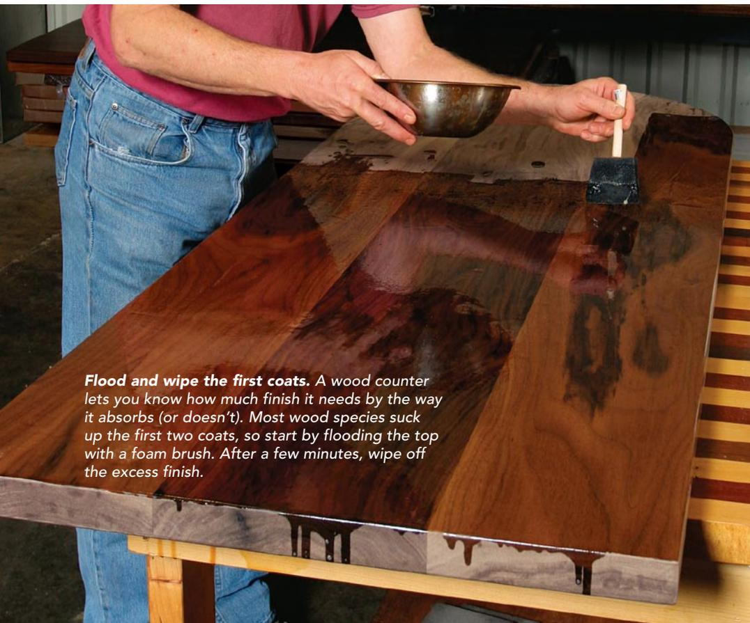
**Flood and wipe the first coats.** A wood counter lets you know how much finish it needs by the way it absorbs (or doesn't). Most wood species suck up the first two coats, so start by flooding the top with a foam brush. After a few minutes, wipe off the excess finish.
