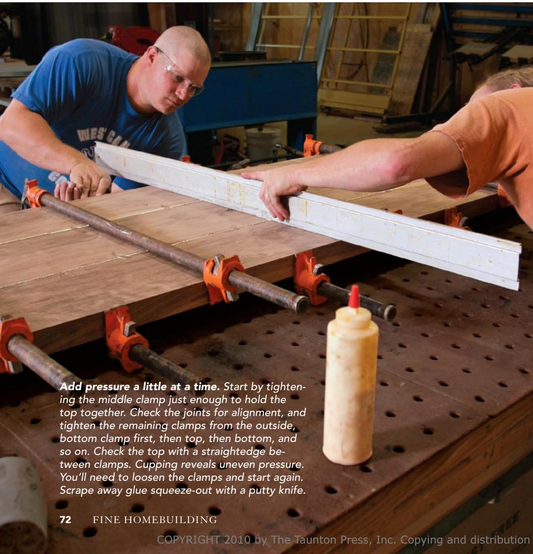
**Add pressure a little at a time.** Start by tightening the middle clamp just enough to hold the top together. Check the joints for alignment, and tighten the remaining clamps from the outside, bottom clamp first, then top, then bottom, and so on. Check the top with a straightedge between clamps. Cupping reveals uneven pressure. You'll need to loosen the clamps and start again. Scrape away glue squeeze-out with a putty knife.
