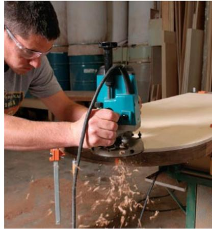
**Make shapes and cut-outs with a template.** First, use the template to trace the shape on the top. Rough-cut the shape with a jigsaw; then use the template again to guide a router and pattern bit to shape the top. Use the same process for sink cutouts, but work with the top upside down. This way, you can screw the template to the top.
