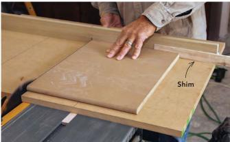
SHIM FOR OUT OF SQUARE If the cut on a board needs to be slightly out of square, slip a shim behind the work until the cut line is parallel with the saw kerf on the sled before cutting.
