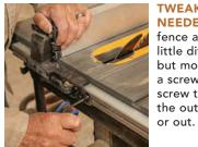
TWEAK AS NEEDED Every fence adjusts a little differently, but most have a screw or Allen screw to adjust the outfeed in
