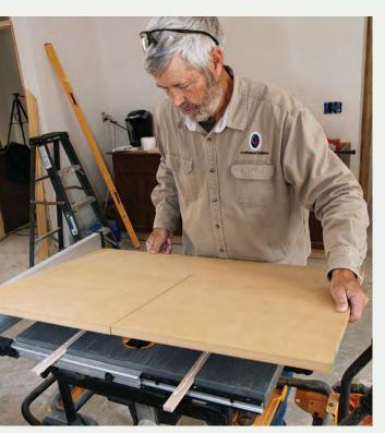
Place the strips in the miter slots, and after applying a bead of glue to them, drop the table into position using the stationary saw blade to align the table.
