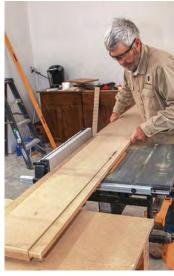
TACK THE WORK TO THE SLED JIG With this option, the work attaches directly to the shelving stock with small nails or screws for making a tapered rip.
