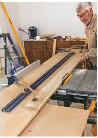
CLAMP-TRACK RIPPING The simplest sled jig for making long tapered rips uses a section of clamp track tacked to the shelving stock. Clamps in the track hold the work in place as you line up the cut with the edge of the sled.
