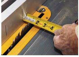
**SET THE WIDTH OF THE CUT** To set the fence position, measure the width of the required cut to the outside of the blade.
