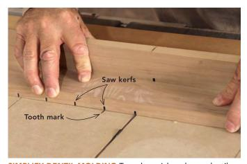
SIMPLIFY DENTIL MOLDING To make quick and easy dentil molding, mark the width of a "tooth" on the sled table out from the blade and set the blade height. Then line up the saw kerfs with the mark for each successive cut.
