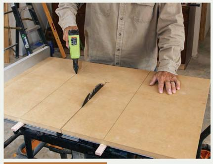
With lines drawn to guide the nail placement, drive brads to attach the table to the strips. Flip the sled table over and hammer the strips tight to the underside of the table to fully engage the brads while the glue sets up.
