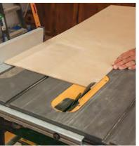
FLAT-OUT APPROACH Always keep material flat against the saw table when feeding it into the blade.
