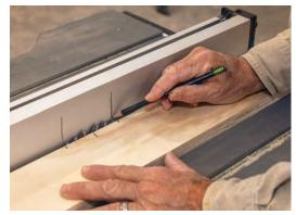
MARK THE BLADE LOCATION With the saw turned off, center a hinge location on the raised blade and transfer the marks to the fence.
