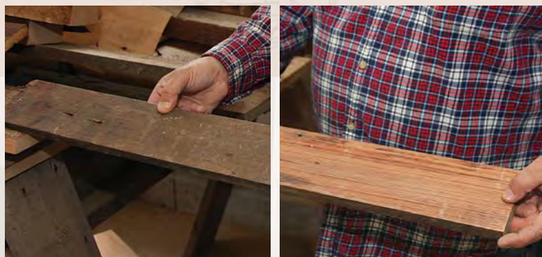
A PEEK INSIDE OLD WOOD When first removed, old wood can appear dingy and uninteresting (left), but a quick pass through the planer can uncover rich, clear grain (right).
