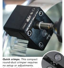
Just insert it into your impact driver and walk it around the perimeter of the pipe.
