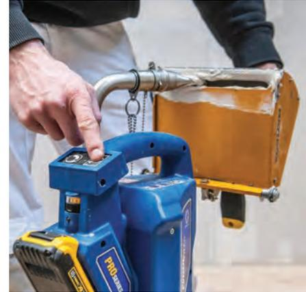
**Press, fill, repeat.** When you need to fill the same tool over and over, the Precision Fill feature allows you to easily program the amount to dispense with one push of a button.
