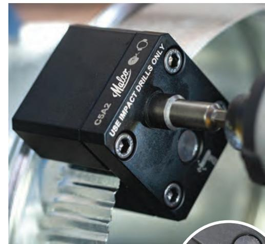
**Quick crimps.** This compact round-duct crimper requires no setup or adjustments. Just insert it into your impact driver and walk it around the perimeter of the pipe.
