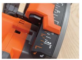
**FAVORITE FEATURE** The depth adjusts in 1/16-in. increments and auto-locks at the desired setting.
