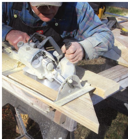
Beam Saw with a swing table. This cut can also be made on a 10-in. tablesaw. You'd need to set the saw to the complement of 61°, which is 29°, and run the material through on edge.
