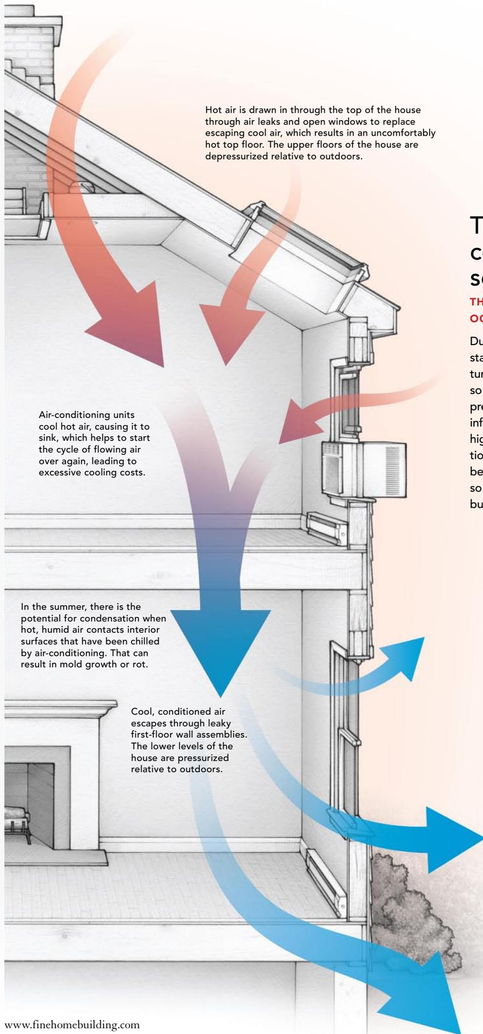
Hot air is drawn in through the top of the house through air leaks and open windows to replace escaping cool air, which results in an uncomfortably hot top floor. The upper floors of the house are depressurized relative to outdoors.
