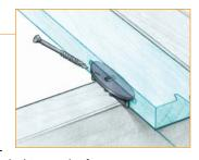
agonal screw attaches both the EB-TY fastener and the leading edge of the decking to the frame.
