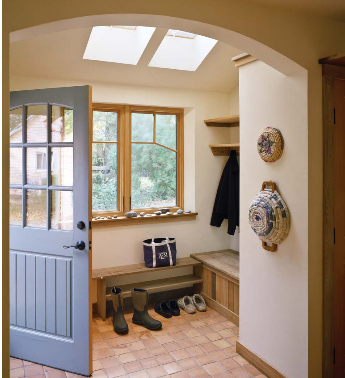
The best room in the house. Built in place of the former enclosed porch, the mudroom's tile floor and well-ordered storage keep the rest of the house free of sand, dirt, and outerwear. Double skylights and windows brighten the 50-sq.-ft. space. Photo taken at C on floor plan.
