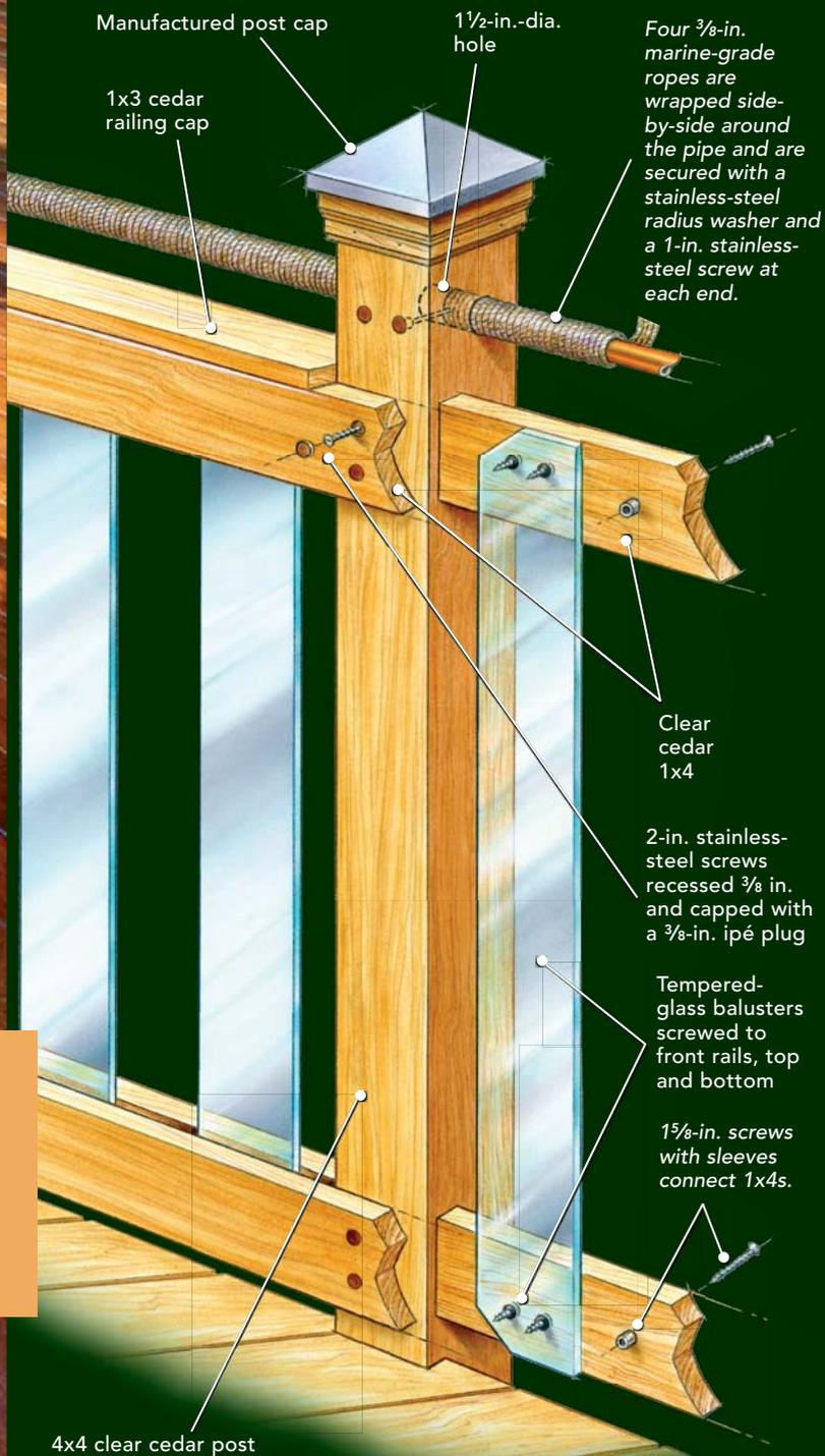
**Cost:** Materials for the glass sections totaled about \$50 per lin. ft. (compared to about \$42 for the aluminum sections). In both cases, the option of using balusters from a manufacturer outweighed the labor cost of fabricating them. Jellema also estimates the choice of clear cedar rather than STK (select tight knot) added about \$6 to \$8 per lin. ft.
