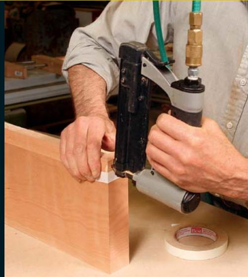
**Frieze: wide, mitered returns.** Glue the returns to the miters, using tape to hold each piece in alignment, then fasten the joint with a couple of pin nails.
