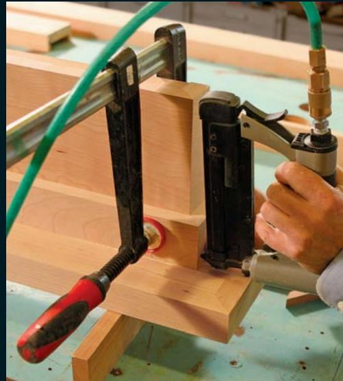
**Add simple layers of trim.** With the shelf-and-frieze assembly turned upside down, dry-fit the two smaller layers of trim, then apply glue, clamp in place, and use a few pin nails to secure the miters.
