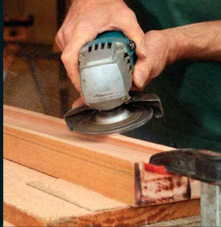
**Sneak up on the scribe.** After clamping the leg onto a worksurface, use an angle grinder equipped with a chainsaw carving blade. Check the fit, and adjust the scribe as needed.
