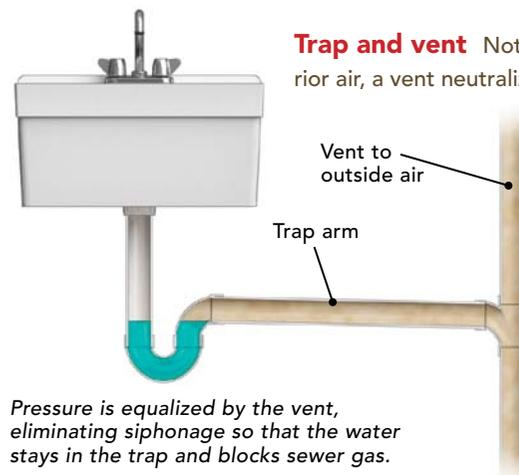
**Trap and vent** Nothing more than a connection to exterior air, a vent neutralizes air pressure within the drain lines. This neutral pressure can be achieved with lots of different configurations: an empty (dry) pipe that connects to the top of a trap arm like a snorkel, a waste (wet) pipe that is oversize in order to provide enough room for both water and airflow, and variations on these setups.
