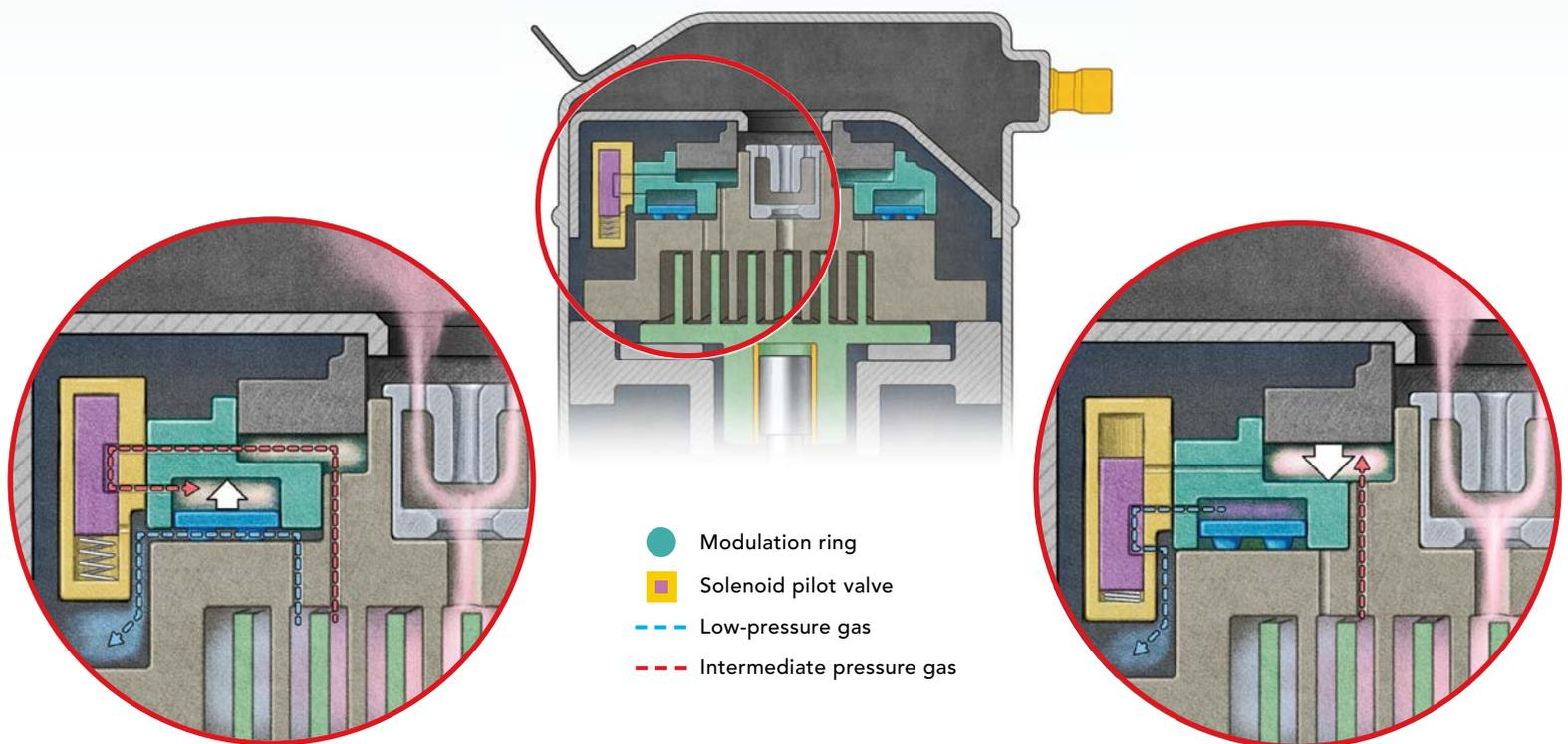
**Partial capacity** The compressor's capacity is controlled by the solenoid pilot valve, which diverts pressurized gas to open or close the scroll's bypass ports in response to signals from the home's thermostat.
