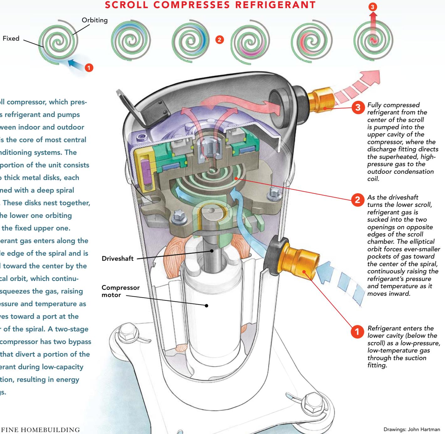
A scroll compressor, which pressurizes refrigerant and pumps it between indoor and outdoor coils, is the core of most central air-conditioning systems. The scroll portion of the unit consists of two thick metal disks, each machined with a deep spiral cavity. These disks nest together, with the lower one orbiting inside the fixed upper one.
