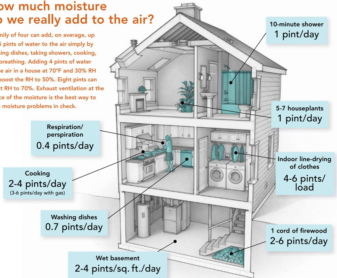
tially drops. No condensation can occur if the air is heated up. However, once the outdoor air is in the house, moisture is added to the indoor air but the temperature of the house stays the same. Hence, the relative humidity and the absolute moisture content rise. How do you add moisture to the air? You breathe, sweat, boil water, take hot showers, and grow houseplants.
