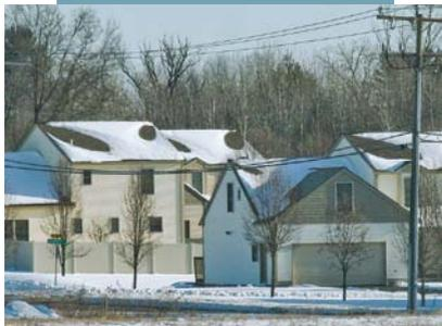
The wind that pushes air into one side of a house also sucks it out the other side. If the outdoor air is moister than the indoor air, water can be driven into framing on windward sides. On a gusty winter day, the pattern of wind pressure can be seen as swirls around corners and edges that sweep snow from specific areas. It is important to have good air-barrier details where roofs, walls, floors, and foundations meet.
