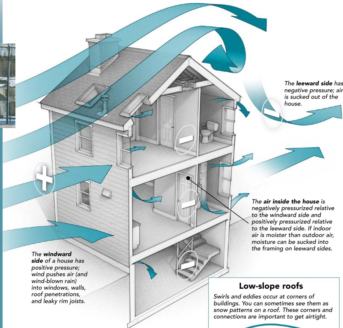
**The windward side** of a house has positive pressure; wind pushes air (and wind-blown rain) into windows, walls, roof penetrations, and leaky rim joists.
