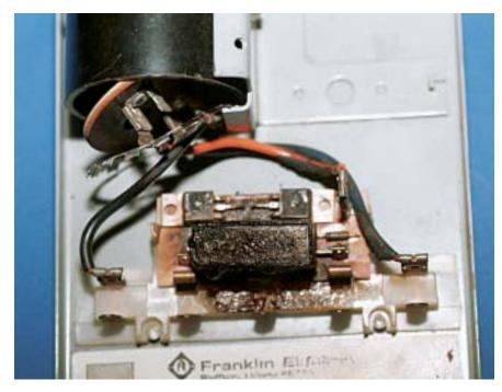
This burned hulk is what's left after a surge came in backward from a well. The surge-protection system within the pump protected the motor but not the control box (the surge also burned out the pressure switch). I've seen the lids of these boxes explode across a room.
