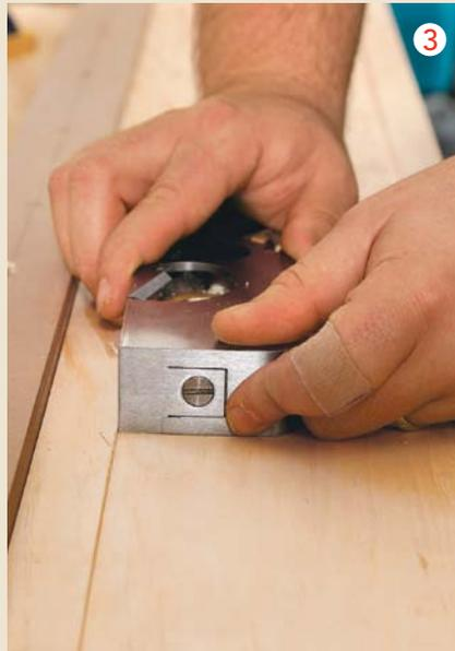
**Clean up the bearing surface.** Use the shoulder plane to smooth the dadoed area. Then turn it on its side, and square up the perimeter edges.
