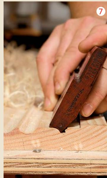
**Hollows cut rounds.** Working from the outer groove, create the rounded portion of the profile with the hollow plane.
