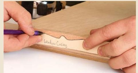
**Plan stock removal.** Once the profile has been traced onto card stock, cut out the silhouette, and trace it onto the trim stock. It's an easy way to see where the most stock can be removed with power tools and where hand planes are most valuable.
