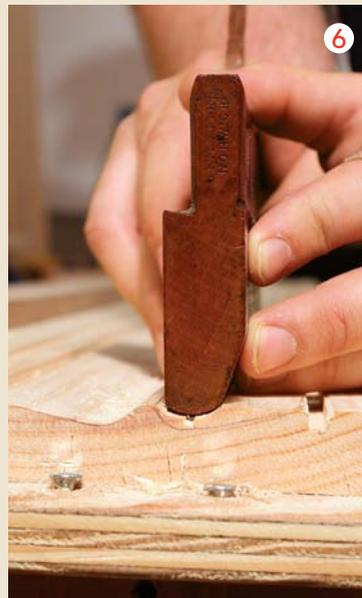
**Rounds cut hollows.** With the inner groove as a guide, use the round plane to cut the dip on each side of the center rib.
