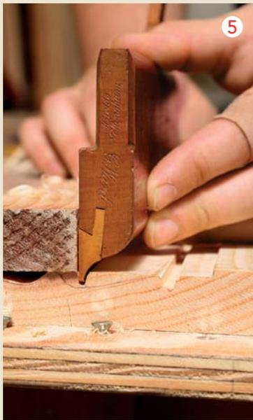
**Define the inner lines.** Set a fence on the stock, and make passes with a snipe's bill plane to the depth of the profile.
