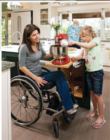
The perfect mix. A mixer lift promised to be a big help in the kitchen, but mounting the hardware on the cabinet sides would require a space-hogging swinging door. The answer: A false wall inside the cabinet that also creates a pocket for a retractable door.
