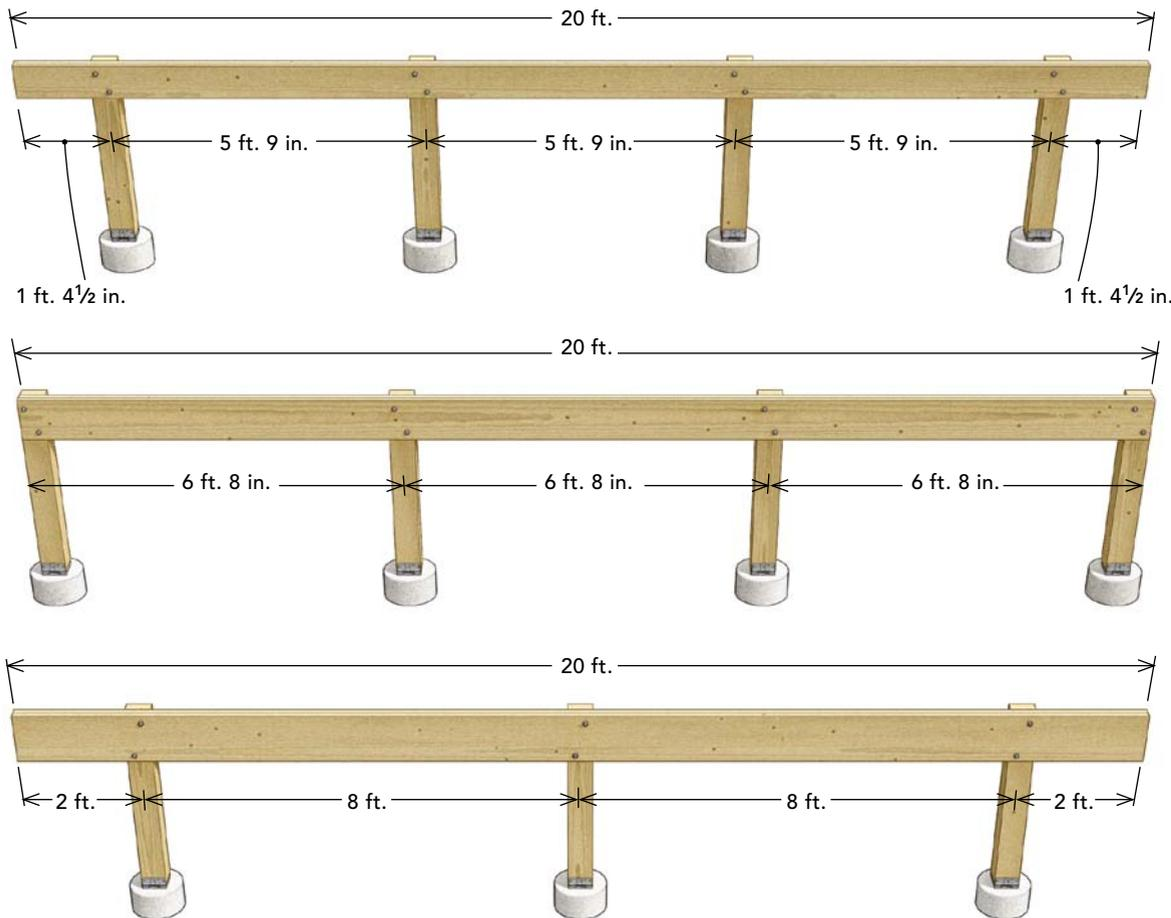
**A double 2x8 beam** offers a maximum span of 5 ft. 9 in. and a maximum overhang of 1 ft. 5¼ in., resulting in four posts spaced 5 ft. 9 in. apart and overhangs of 1 ft. 4½ in. at the ends.
