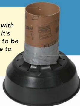
**Tapered tube.** The Footing Tube includes a concrete-saving tapered plastic tube in addition to the bell-shaped footing form. It offers little bite for ice to grab and lift, and it allows backfill to be compacted prior to placing the concrete.
