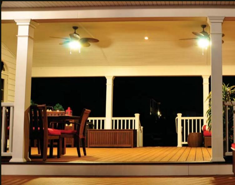
**Dining lights should be overhead.** Porch roofs and pergolas provide the ideal location for line-voltage-connected dining fixtures and ceiling fans. The roof makes it easy to hide the wires and provides a sturdy spot for mounting the fixtures. Lighting for dining areas should be dimmer controlled to match the mood.
