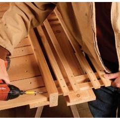
Fasten into the end grain. Align the end of the lattice panel with the end of the center rail assembly, and then drive 2<sup>1</sup>/4-in. stainlesssteel screws through the 2x4 into the end grain of the lattice uprights.
