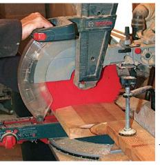
Cut the caps to length. Using a stop to ensure consistency, cut the board into 8-in. caps on a miter saw. Do not raise the blade after finishing the cut until it has stopped completely. Otherwise, the blade is likely to jam on the cut cap.
