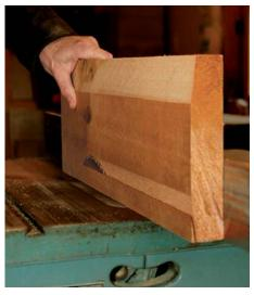
**Bevel a full board.** Rip the stock to 8 in. wide, and then cut the bevels along the two long edges of the board. This saw's blade tilts right, so the cuts had to be made with the fence to the left of the blade.
