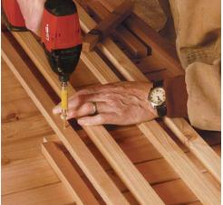
Space the center uprights after assembling the ends. Cut a 17<sup>5</sup>/8-in.-long gauge block to set the next pair of uprights relative to the first pair. Again, use the small gauge blocks to create a 1-in. gap between the pair of uprights.
