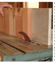
Gang-cut the end-grain bevels. Rip a long scrap of plywood to the same width as the caps. Secure the caps to the plywood with screws driven through the back side. Position the tablesaw fence to match the thickness of the plywood, and run the whole setup through the saw to bevel the end grain of the caps.
