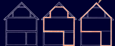
Pencils down. To be effective, air barriers must be continuous. Tracing the location of the air barrier without lifting your pencil on a set of cross-section drawings is a good test. Unfortunately, most construction drawings omit air-barrier details or even where the air barrier is located.
