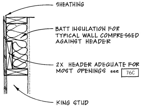
The goal when designing an energy-efficient header is to allow for the most insulation while providing for nailing at both the exterior and interior of the opening.
