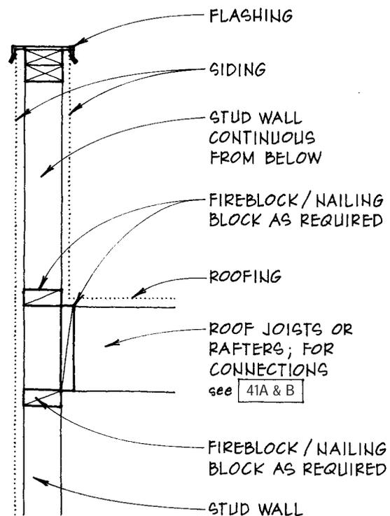
**D** PARAPET WALL FRAMING ROOF JOISTS SHOWN ⊥ TO WALL
