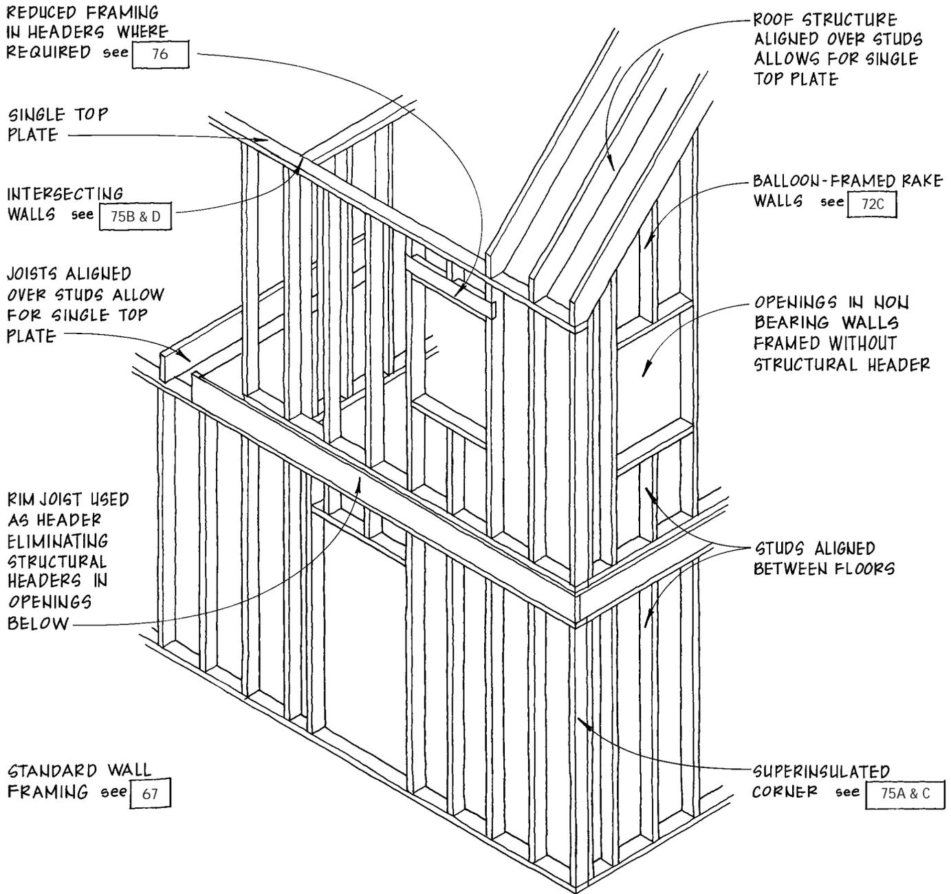
**Advanced framing**—Advanced framing minimizes the amount of framing that spans from the interior to the exterior of a wall, thus lowering the effect of thermal bridging. By limiting the amount of framing, more volume in the wall can be occupied by insulation, which increases thermal performance of the overall assembly. Advanced framing alone can
