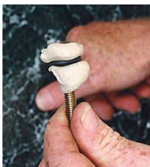
Tank bolts tie the two-piece toilet together.
